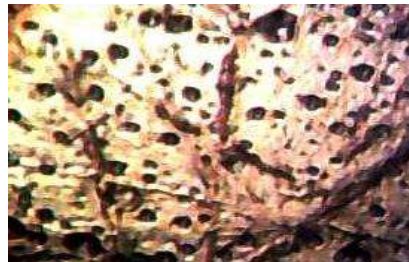
Figure 4 — Photographs of the sample surface (W -1), after irradiation (irradiation dose 5 \times 10^{17} ion/cm 2 ).
