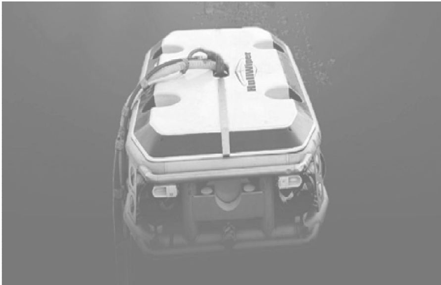
Picture 2 – The underwater hull cleaning machine
