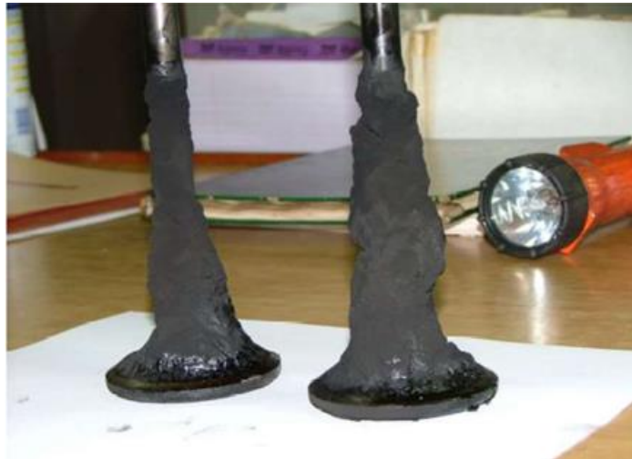
Figure 4. Incompatibility and instability of residual fuel
