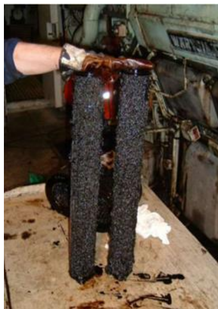
Figure 5. Incompatibility and instability of residual fuel
