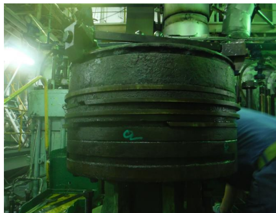
Figure 7. Piston crown with broken and missing rings due to Cat Fines
