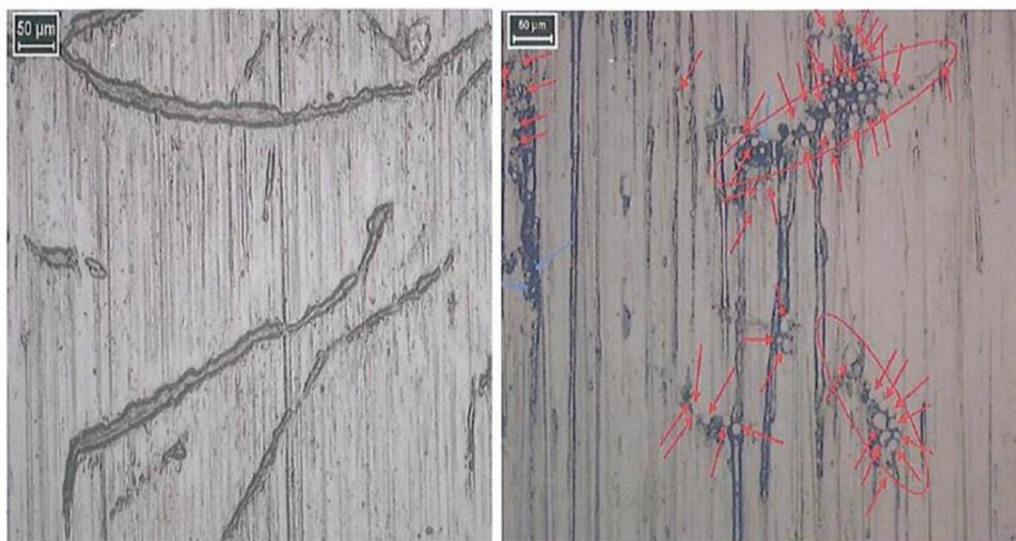
Figure 2. A magnification of cylinder liner walls showing typical accelerated wear marks due to Cat Fines and a cluster of Cat Fine particles embedded in the surface
