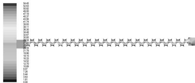
Figure 2 – Velocity of exhaust gases in the channels of tube bundles with shifting, m/s ( Re = 18,6 \cdot 10^3 )
