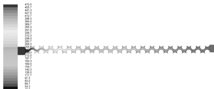
Figure 3 – Change of temperature in the channels of tube bundles with shifting, °C ( Re = 18,6 \cdot 10^3 )
