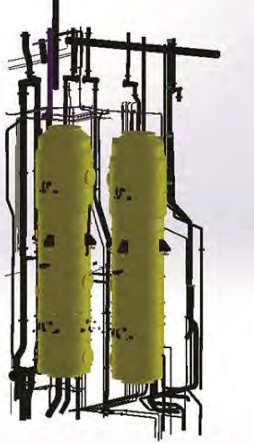
Figure 6. A 3D model of the scrubber with system connections.
